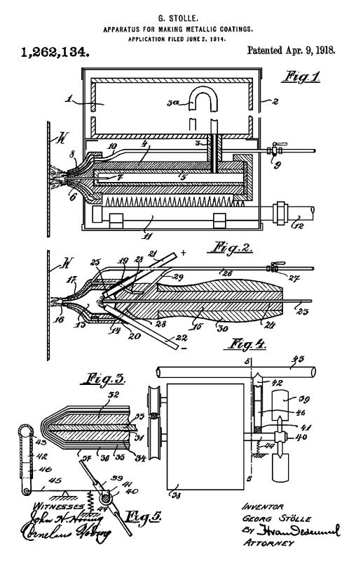
In the form of construction shown in Fig. 2, the volatilizer 13 is constructed in the front end 14 of a holder 15 provided with a handle 30. At the front end of the volatilizer 13 a volatilizing nozzle 16 is arranged which projects beyond the suction nozzle 17 in similar manner to what was the case in Fig. 1. In the arrangement shown in Fig. 2, arc-light carbons 21 and 22 serve
